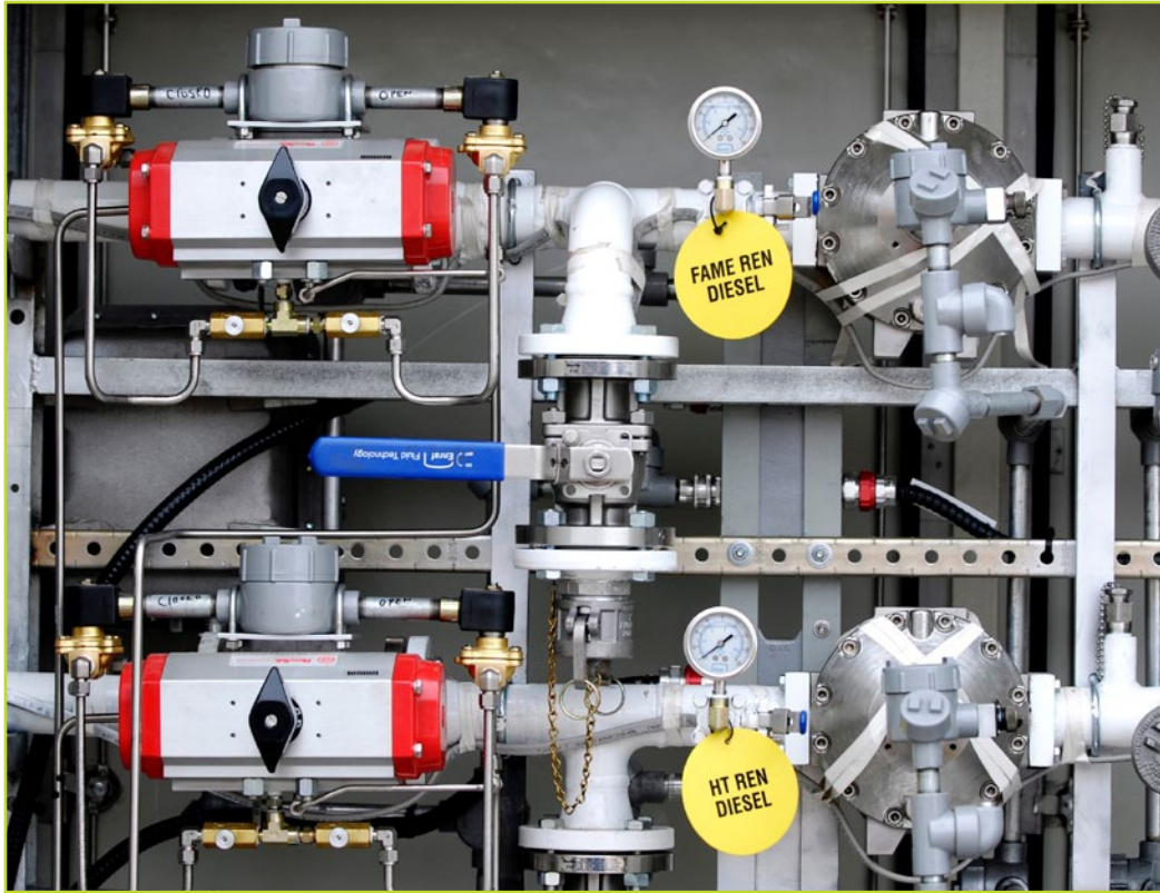
FIGURE 11: Close-Up of Micro-Blenders for FAME and HT Fuels
